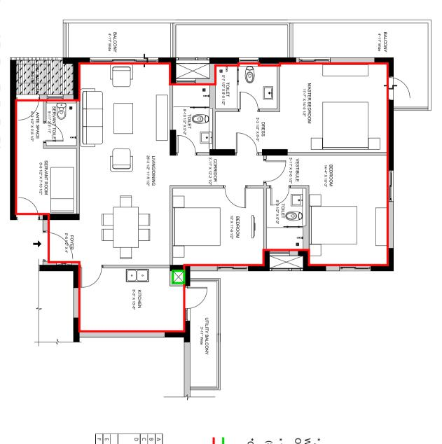
\* APPROX. INTERNAL DIMENSIONS CLEAR OF MASONRY WORK,LOSS OF 2.5-4.0 CM IS EXPECTED ON ACCOUNT OF PLASTER, SKIRTING & OTHER FINISHES.
