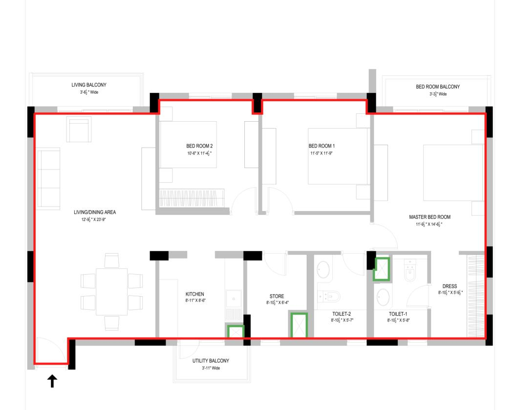
\* APPROX. INTERNAL DIMENSIONS CLEAR OF MASONRY WORK, LOSS OF 2.5-4.0 CM IS EXPECTED ON ACCOUNT OF PLASTER, SKIRTING & OTHER FINISHES.
