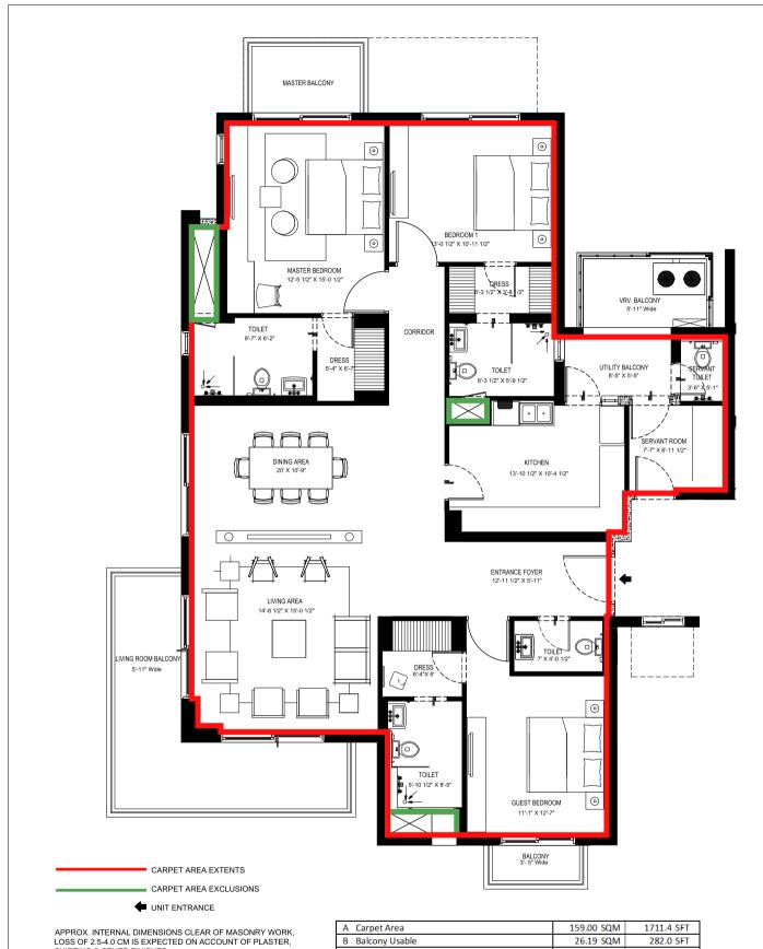
APPROX. INTERNAL DIMENSIONS CLEAR OF MASONRY WORK, LOSS OF 2.5-4.0 CM IS EXPECTED ON ACCOUNT OF PLASTER, SKIRTING & OTHER FINISHES.
