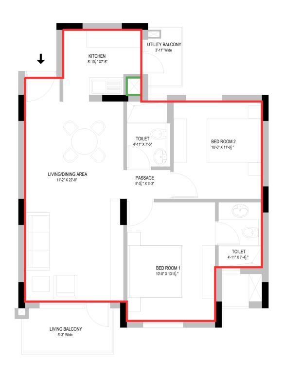
\* APPROX. INTERNAL DIMENSIONS CLEAR OF MASONRYWORK,LOSS OF 2.5-4.0 CM IS EXPECTED ON ACCOUNT OF PLASTER, SKIRTING & OTHER FINISHES.
