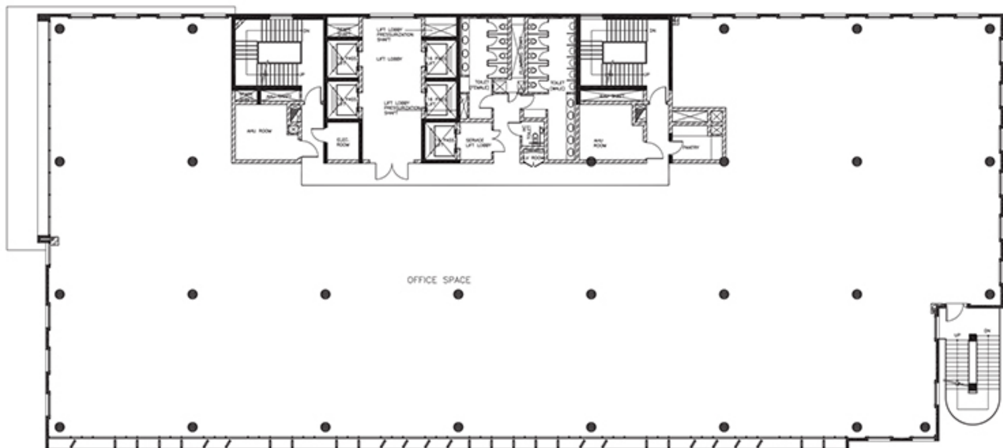
TYPICAL OFFICE FLOOR PLAN - BLOCK C
